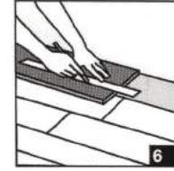
Door frames and heating vents also require expansion room. First cut the plank to the correct length. Then place the cut plank next to its actual position and use a ruler to measure the areas to be cut out and mark them. Cut out the marked points allowing them the necessary expansion distance on each side. **Diagram 7.**
